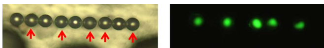
Fig. 6. (Left) Bright field and (right) fluorescence micrographs of microstamped 40- \mu\text{m} beads. The arrows indicate beads stamped by FITC-BSA.
