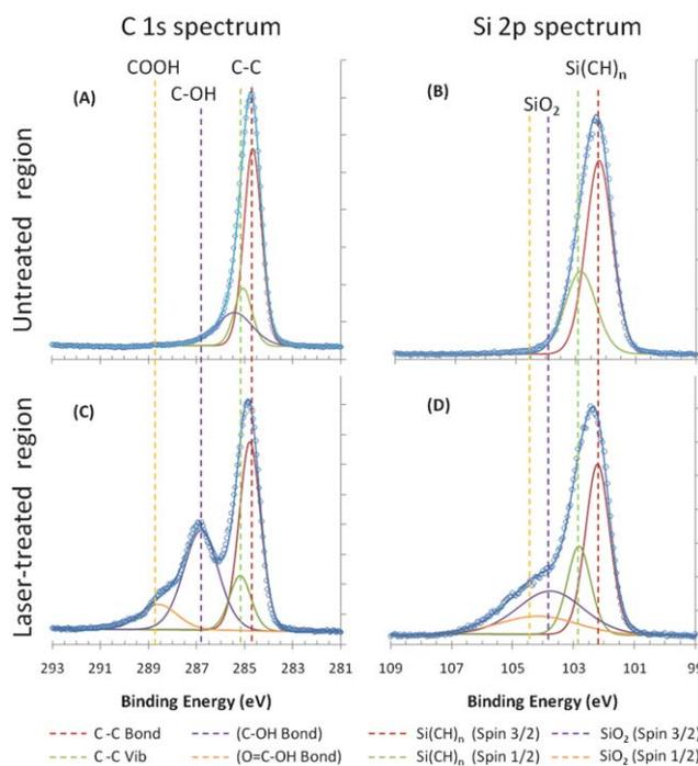
**Fig. 4** XPS surface analysis high resolution spectra; (A) untreated region C 1s spectrum, (B) untreated region Si 2p spectrum, (C) laser-treated region C 1s spectrum, and (D) laser-treated region Si 2p spectrum.
