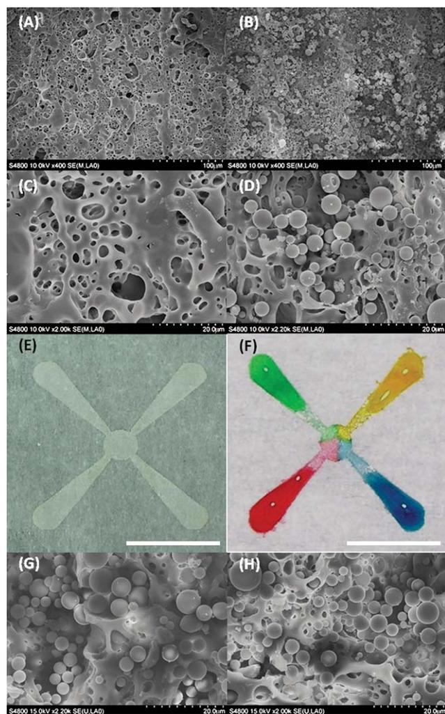
**Fig. 5** Silica microparticle deposition on laser-treated areas; (A and C) SEM of a laser-treated area without microparticles, (B and D) SEM of a treated area with microparticles, (E) pattern after silica particle deposition, (F) colored water diffusing towards the center after droplets were placed in the corners (scale bar: 10 mm), (G) SEM of dried sample after water flow, and (H) SEM of dried sample after testing under water.
