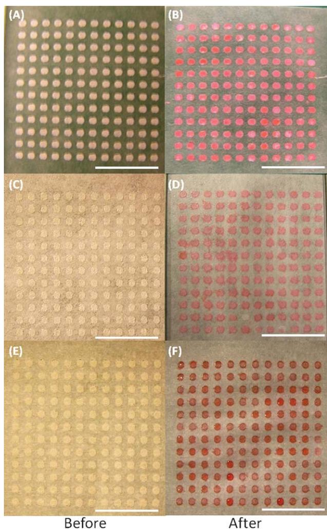
**Fig. 2** Comparison of laser treatment on various hydrophobic papers before and after dipping in aqueous red dye. (A and B) Wax paper, (C and D) palette paper, and (E and F) parchment paper. (Scale bar: 10 mm; red dye was added to improve the contrast.)
